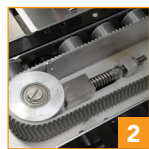
Self-tensioning & self-tracking drive belts simplify belt replacement
