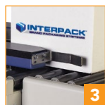
Stainless steel self-centering in-feed guides for simple case size setup
