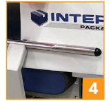
Arcing self-centering guides for simple case size setup
